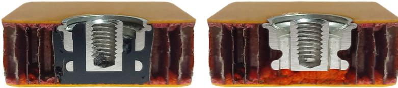
Another advantage of the **SECAMnida®**: its weight. The insert is made of an aluminium alloy combining strength and cold forming properties for crimping, with reinforcement of the interior threads and the addition of a stainless-steel threaded insert to achieve the best mechanical strength/weight ratio.
