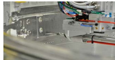
Chamfering after machining of bores and edges
