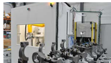
Robotic deburring cell
