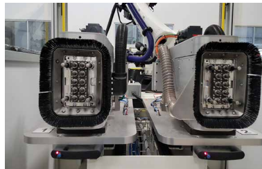
► Automatic effector exchange for manual drill bit replacement.
