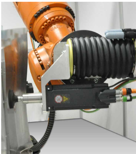
◄ Polishing machining grooves on titanium
